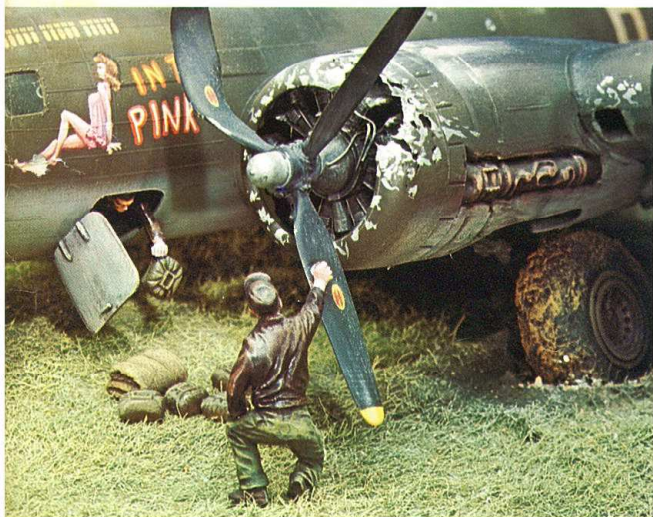
Flak damage and a resulting fire forced the crew to shut down the number two engine. The feathered prop can be duplicated by cutting the blades where they meet the spinner, and rejoining them as shown. To duplicate flak damage and shell holes, carefully use a hobby grinder to thin out the cowling, fuselage, and any other panels you may wish to depict as being damaged.
