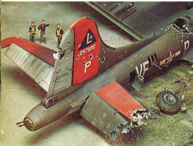
The flak-ravaged tail surfaces were formed by carefully grinding the styrene on the back side before assembly, and then cutting the thin remaining wall of styrene to resemble jagged metal. Remember, if major damage is attempted, as shown on the horizontal stabilizer, that some interior details must be added. Note that the B-17 control surfaces were fabric-covered, and would not be jagged after they were damaged.
